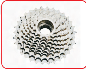
SBD-MF901 INDEX 9-SPEED , TEETH-12T-32T THREAD-1.375X24TPI , FINISH-BLACK/BROWN/CP
