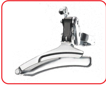
SBD-FD02 FRONT DERAILLEUR FRICTION DOWN PULL SUITABLE FOR DOUBLE CHAINWHEEL, STEEL CLAMP DIA-28.6MM, TOP GEAR-48T, CAPACITY-14T FINISH-CP/UCP/ED
