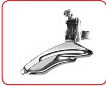
SBD-FD04A FRONT DERAILLEUR FRICTION TOP PULL SUITABLE FOR 24/21 SPEED, CLAMP DIA- 28.6MM/31.8MM TOP GEAR-48T, CAPACITY-22T FINISH-CP/UCP/ED
