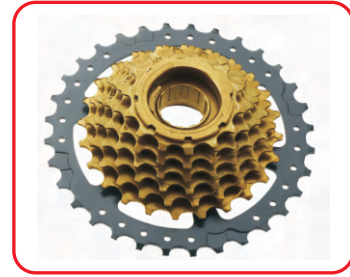
SBD-MF702 INDEX 7-SPEED , TEETH-14T- 32T THREAD-1.375X24TPI , FINISH-BLACK/BROWN/CP
