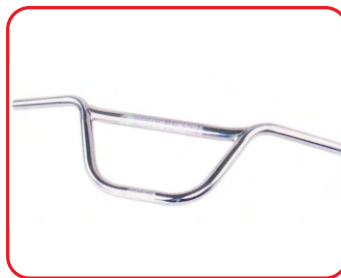
SBD-HB08 HANDLE BAR BRAZILIAN TYPE WIDTH-600-680MM RAISE-180MM MATERIAL-STEEL
