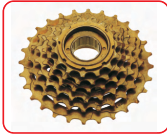
SBD-MF611 INDEX 6-SPEED , TEETH-14T-28T THREAD-1.375X24TPI , FINISH-BLACK/BROWN/CP
