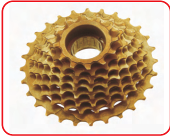
SBD-MF801 INDEX 8-SPEED , TEETH-12T- 28T THREAD-1.375X24TPI , FINISH-BLACK/BROWN/CP
